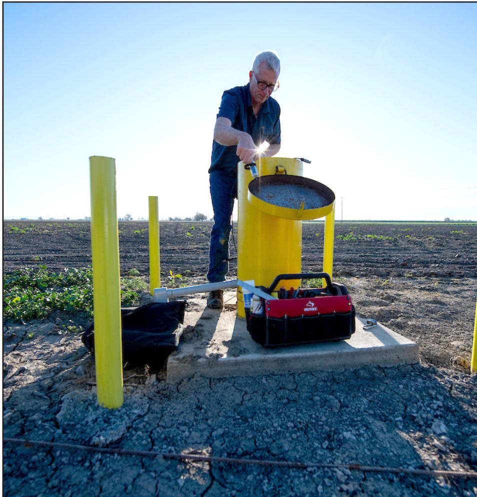
An engineering geologist with the California Department of Water Resources, measures groundwater levels at designated monitoring wells in Yolo County.
